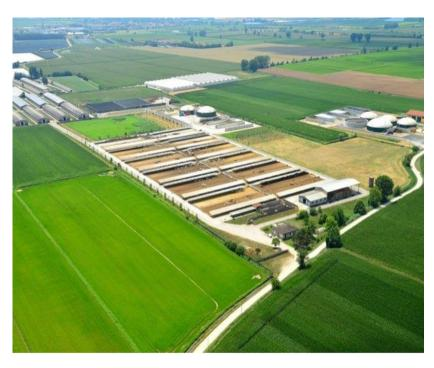
Example of Biogasdoneright in action: Cooperativa La Torre: 2 biogas plants of 1 MW electric each. Daily input: 90 tons cow manure, 90 tons cow slurries, 38 tons eggs laying chicken manure, 10 tons rabbit manure, 5 tons spent mushrooms litter, 10 tons sugar beets, 30 tons corn silage, 5 tons rye grass (all wet weights)
